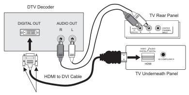
After the connections have been made, tighten the screw to secure the cables.
